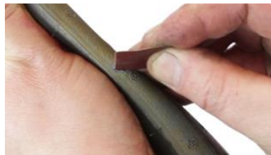
Roughen edges around puncture site with sandpaper,
